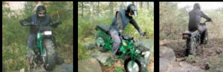
Rokons have 15 inch ground clearance. A steel skid plate protecting the engine allows climbing over larger obstacles. Steep inclines are no problem for a Rokon.
