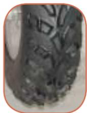
The Titan AT489 is the widest Rokon tire available (8 x 12 x 25). Its unique tire pattern provides optimal off road traction. It is the tire of choice for 12-inch wheels.
